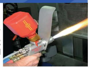
Once metal sprayed, the built-up area can then be ground or machined to very fine tolerances, in order to produce a repaired component which is often better than the original.
